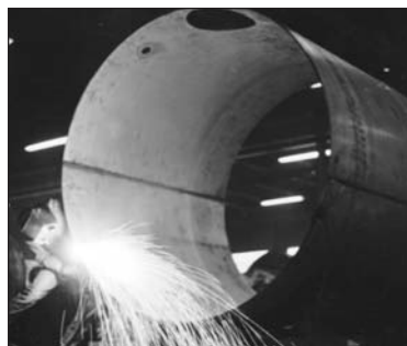
Tank cylinders are automatic TIG welded for superior weld quality.
