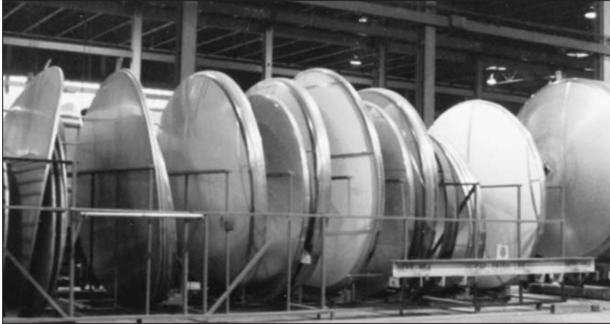
Mueller tank heads range in size from 18 inches to 24 feet in diameter, from 12-gauge to 1-inch thick material.
